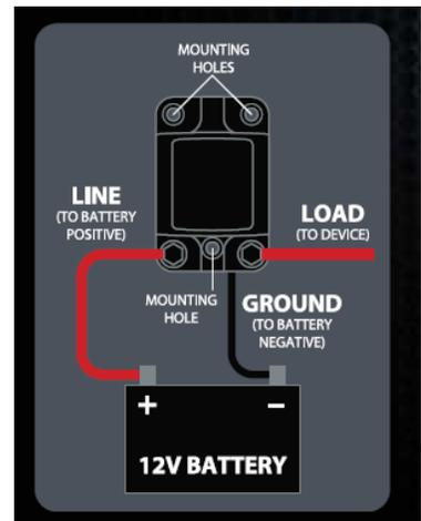
**ATTENTION:** The Breaker's ground wire must be connected to the battery negative for the breaker to function.
